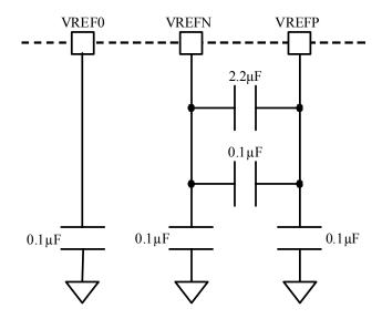
Use laminated ceramic capacitors (capacitance tolerance:  $\pm 10\%$ , temperature coefficient:  $\pm 15\%$ ) or those of higher characteristics except for the 2.2 $\mu$ F capacitor.
