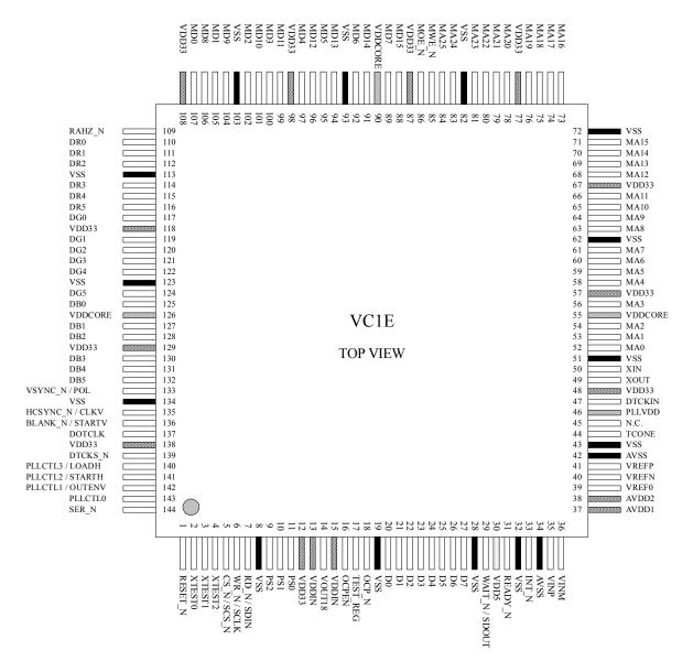
Note: N.C. (pin 45) is a no connection pin, with only lead frame, and no bonding wire is connected.
