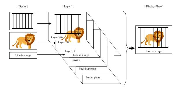
Any one among sprite, two or more lines, and text can be selected in one layer. One sprite, one character string, and lines (up to 510) can be displayed on one layer.
