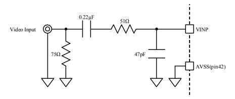
Use laminated ceramic capacitors (capacitance tolerance:  $\pm 10\%$ , temperature coefficient:  $\pm 15\%$ ) or those having higher characteristics.
