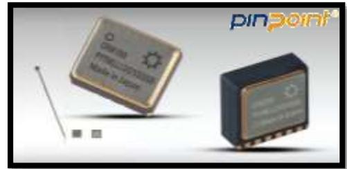
PinPoint® is a tiny (6.3x5.5x2.7mm), yet powerful, surface mountable LCC ceramic packaged, single-axis MEMS angular rate sensor (gyro), capable of measuring angular velocity up to a maximum of  $\pm 1,000^\circ/\text{s}$  which has two output modes; an analogue voltage signal which is linearly proportional to angular speed, and a digital signal in SPI® protocol. The choice of output mode; analogue or digital, is determined by the user when connecting it to the user's host PCB.
