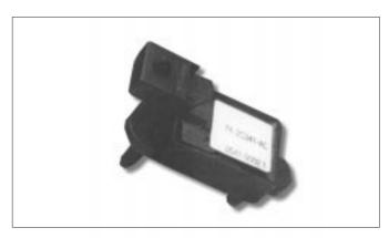
Custom AEC sensors offer a low cost, high reliability alternative to micromachined sensors and mechanical switches for low G-force applications, such as automotive ride control, anti-lock brakes, and passenger safety restraint systems. They are based upon our proven hermetic switch technology, fully encapsulated within custom housings. They respond to G-force in the horizontal plane, from 0.2 to 0.8G per design, and provide normally open, or normally closed contacts per customer requirements.
