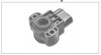
This new electronic analog sensor is capable of continuous operation from -40°C to 150°C and features complete encapsulation of its electronic circuitry. These sensors are designed to replace conventional wiper-contact, resistor-based rotary position sensors where water, vibration and contact wear cause premature failures and contact noise problems.
