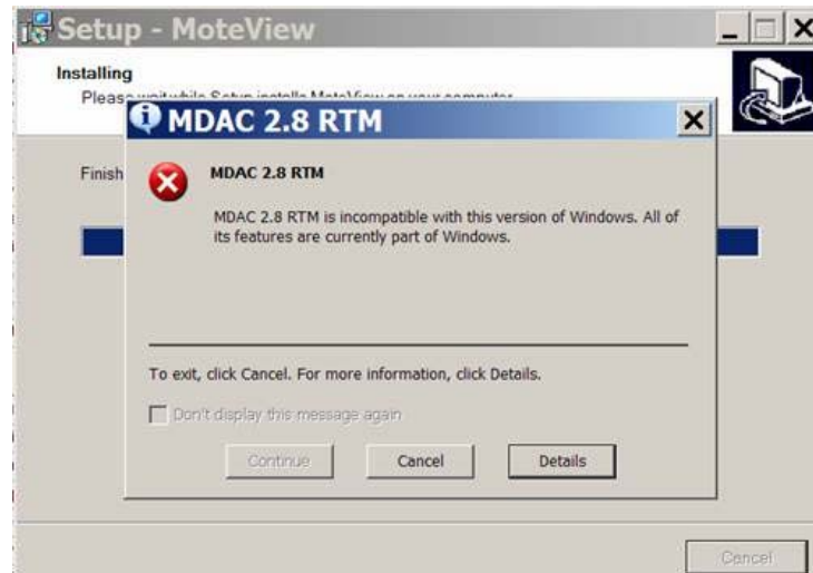
Figure 2-6. MDAC 2.8 RTM incompatibility message that may appear during .NET installation. This warning can be ignored by clicking on Cancel.
