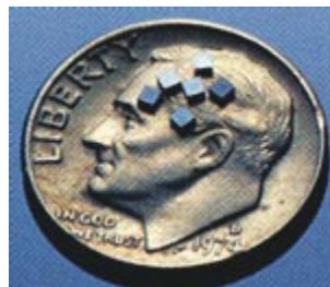
Micromachined Tilt Sensor Element
